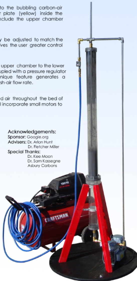
An Open-Brayton Cycle with our Carbon-Particle Dispenser.
