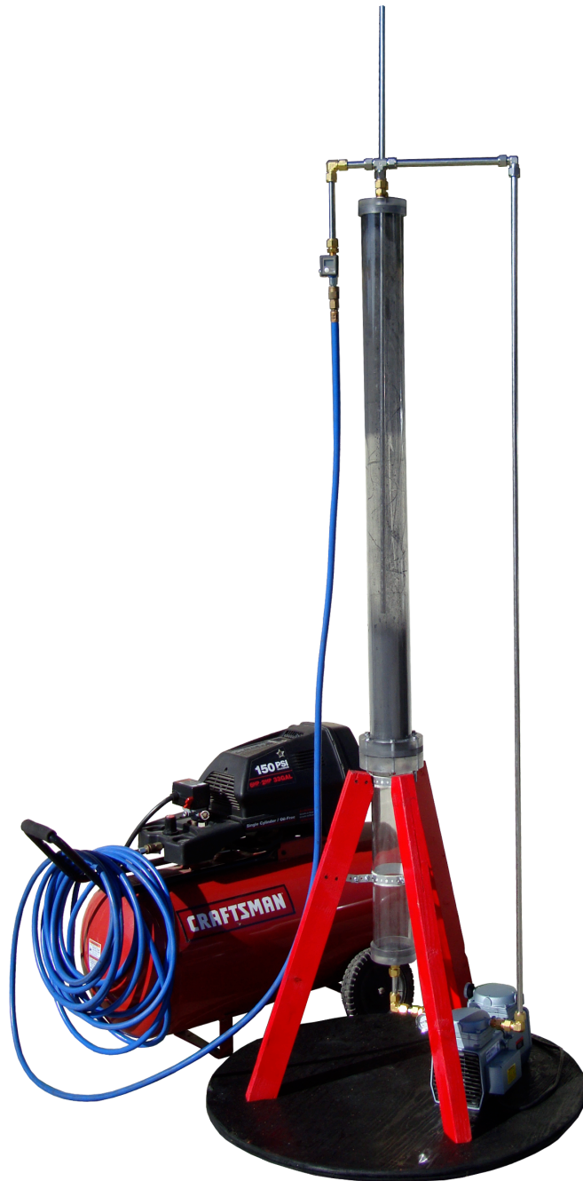
Fig. 11. Carbon Particle Dispenser: Final Design
